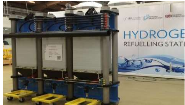
1MW balancing electrolyser
